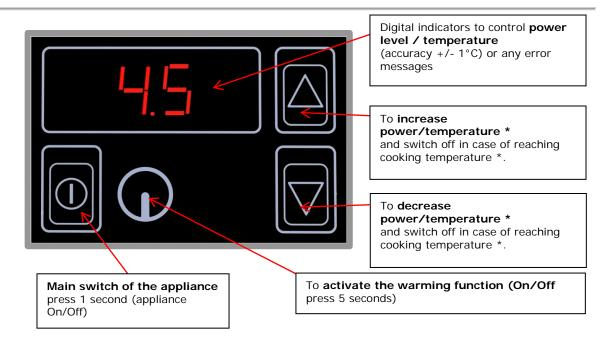
When pressing the keys, an LED light indicates that the command was recognised.
