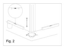
Significant unevenness or inclinations can compromise the operation of the oven.
