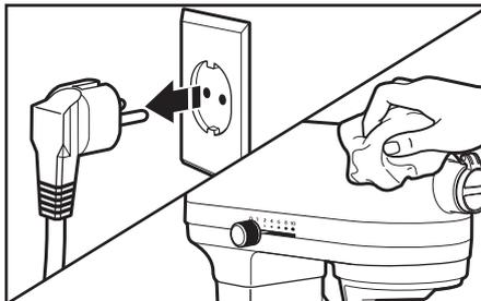
**1** Always be sure to unplug Stand Mixer before cleaning. Wipe Stand Mixer with a soft, damp cloth. Do not use household/commercial cleaners. Wipe off beater shaft frequently, removing any residue that may accumulate. Do not immerse in water.
