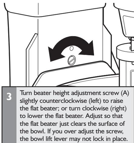
**NOTE:** When properly adjusted, the flat beater will not strike on the bottom or side of the bowl. If the flat beater or the wire whip is so close that it strikes the bottom of the bowl, the coating may wear off the flat beater (for coated beaters) or wires on the wire whip may wear.
