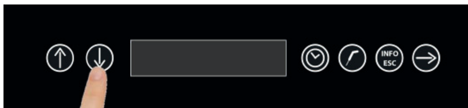
Pressing the UP or DOWN buttons you can scroll the whole menu
