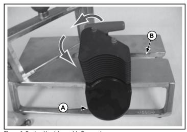
Figure 3. Pusher Head Assembly Removal
