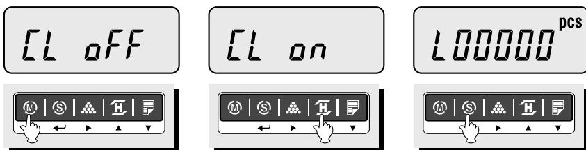
① Press the MODE key until the display shows "CL OFF". It means the counting comparison function is deactivated.
