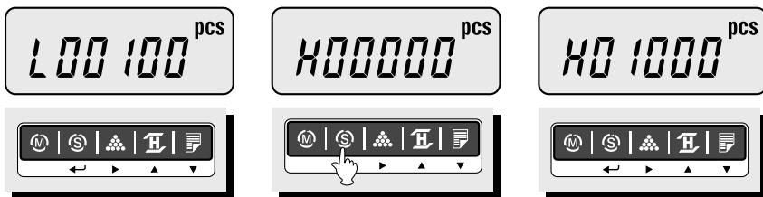
④ Press the HOLD (▲) or PRINT (▼) key to have number up or down. To enter next digit, press the SAMPLE(►) key.
