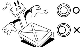
Keep the scale away from other electromagnetic generating devices. This may interfere with accurate reading.
