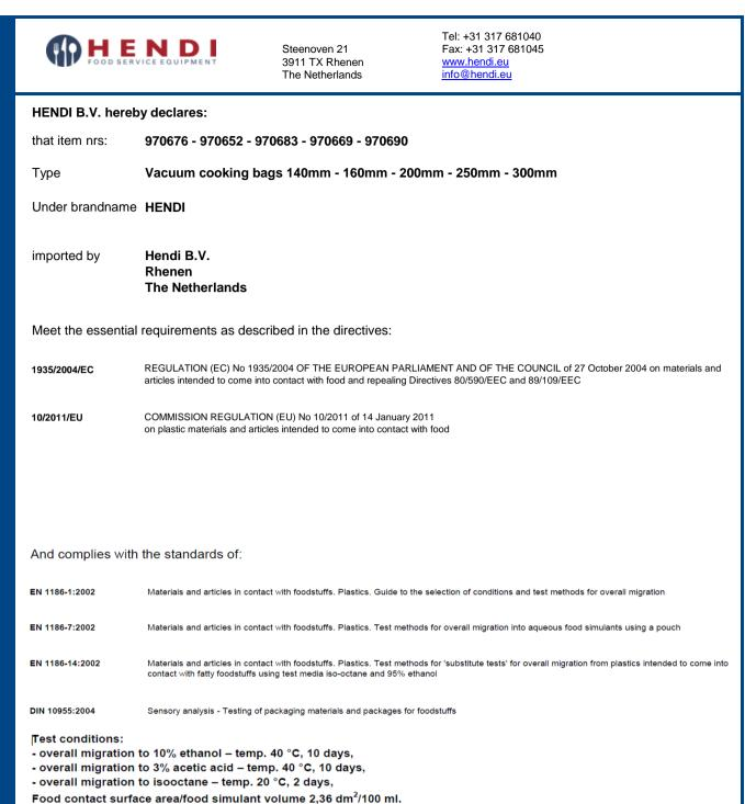
According to 10/2011/EU "Testing for 10 days at 40 °C shall cover all storage times at refrigerated and frozen conditions including heating up to 70 °C for up to 2 hours, or heating up to 100 °C for up to 15 minutes."
